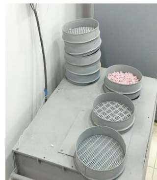
Figure 2. Process of determining the optimal mesh surface of the seed cotton cleaner.
