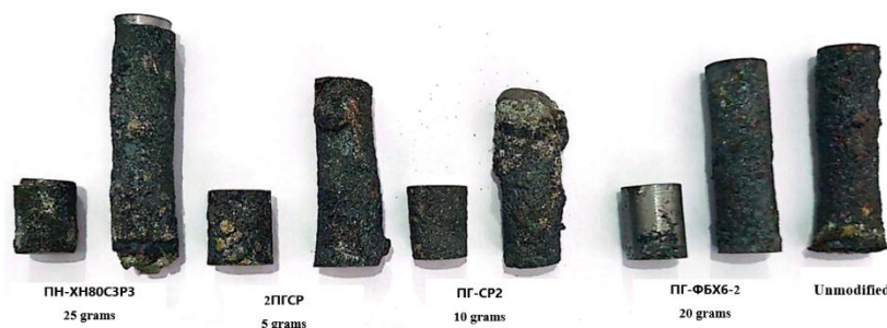
Fig 3. Appearance of cast samples made of 20Л grade steel after sand removal
