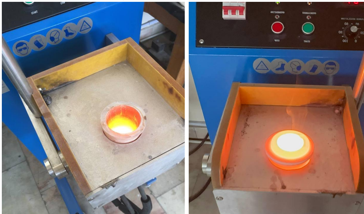
Fig 1. The process of melting charge materials in the IST-0.001 induction furnace
